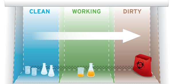
Distribute items evenly in the work area to help maintain uniform airflow. Supplies and equipment (especially aerosol generators such as vortex mixers or tabletop centrifuges) should be as close as practical to the rear of the work area, away from the front grill.
