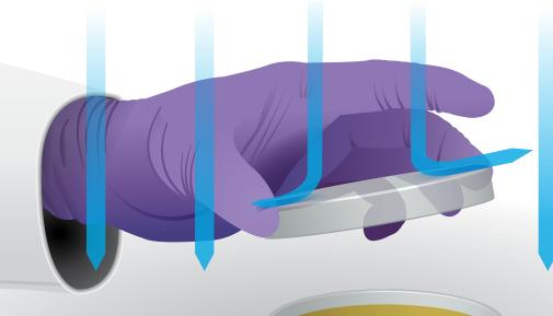
When working with petri dishes and tissue culture plates, hold the lid above the open sterile surface in order to minimize the impaction of air downflow.
