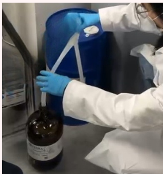
Hand siphon pump for transferring solvent
