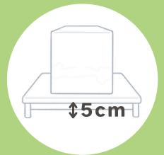
Raise large equipment at least 5 cm above the base to prevent airflow blockages
